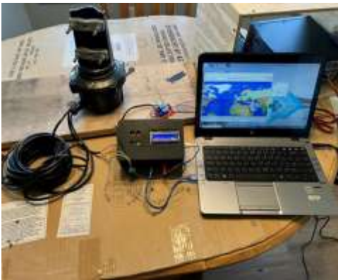
Computer-controlled satellite azimuthal tracking at LabNLunch
