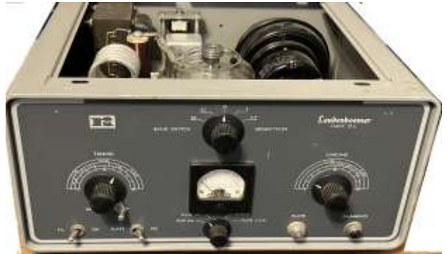
Hallicrafters HT-45 Loudenboomer Single Tube Amplifier
