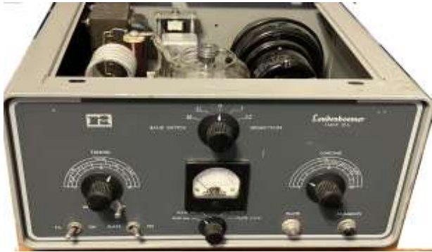
Hallicrafters HT-45 Loudenboomer Single Tube Amplifier
