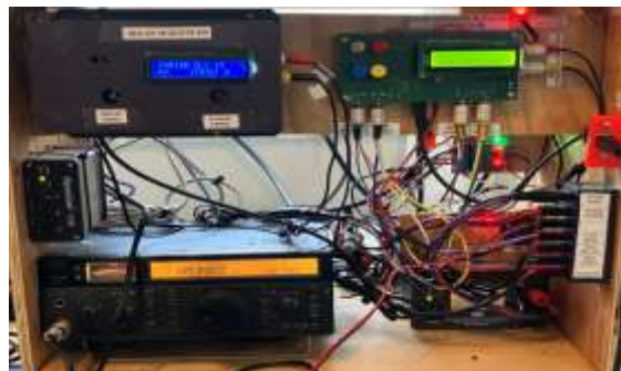
Simple plywood satellite ground station go-box. Ancient radio lower left; homebrew K3NG Arduino Nano rotator controller upper right. Power supplies lower right. Sequencer (upper left) not necessary without preamps. Signalink would allow digital (primarily for tropospheric FT8 at present).
