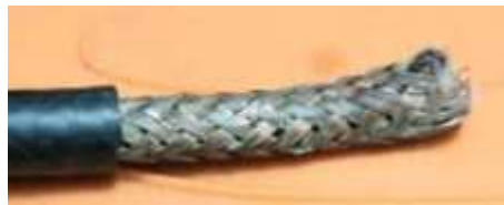
(Left & above) MERT’s technical team (Ray Woody WB6FKJ, Santos Pagan KR4FEP and Roy Sherwood WA9MID) identified several issues at two shelters - Lake Weir High School and Madison Street Elementary on June 9th. Issues included corroded coaxial connectors, water soaked/corroded cable, a broken antenna and indoor coaxial cable used outdoors on the roofs of both schools.
