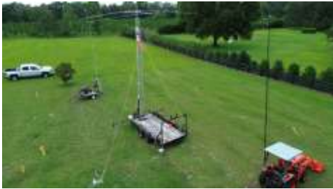
3-band Yagi and 3-element 40m Inv Vee Yagi (masts visible) drone photo by Jim Carr KC4MHH
