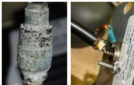
(Left & above) MERT’s technical team (Ray Woody WB6FKJ, Santos Pagan KR4FEP and Roy Sherwood WA9MID) identified several issues at two shelters - Lake Weir High School and Madison Street Elementary on June 9th. Issues included corroded coaxial connectors, water soaked/corroded cable, a broken antenna and indoor coaxial cable used outdoors on the roofs of both schools.
