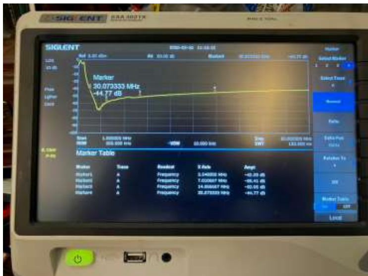
Figure: Common mode rejection of FT-240-31-based filter, from 1-50 MHz, showing roughly 40 dB rejection on 80m and better rejection around 50 dB on higher HF bands. Not quite as good at 80 meters as the FT-240-43 filter, but otherwise fairly similar
