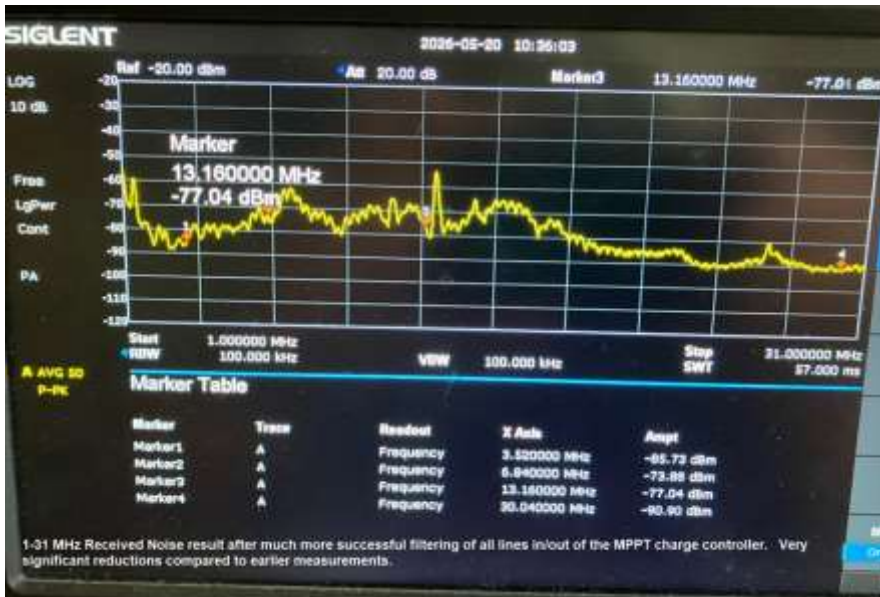
Figure: Much lower noise signatures obtained with filtering of all lines in and out of the MPPT charge controller. Noise signatures are now down in the -70 dBm or below. Stronger peaks probably represent international broadcast stations.
