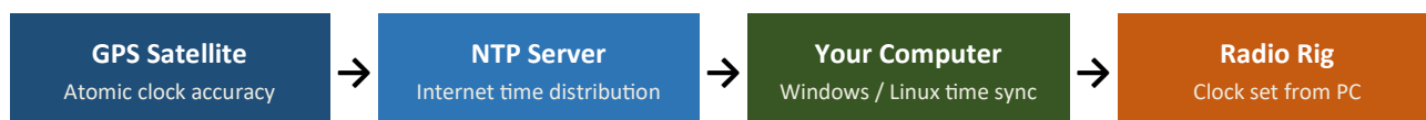
Figure 1 — Time travels from GPS satellites through NTP servers to your computer, then to your radio.
