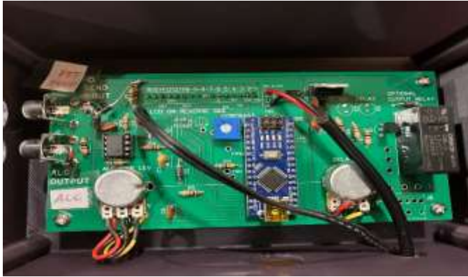
Version 0.1 populated and working prototype board
