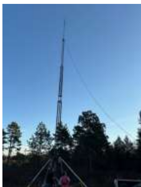
GARS mobile antenna trailer elevated to over 60 feet high
