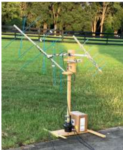
Figure 9: Final antenna setup on homebrew dual-axis rotator system.
