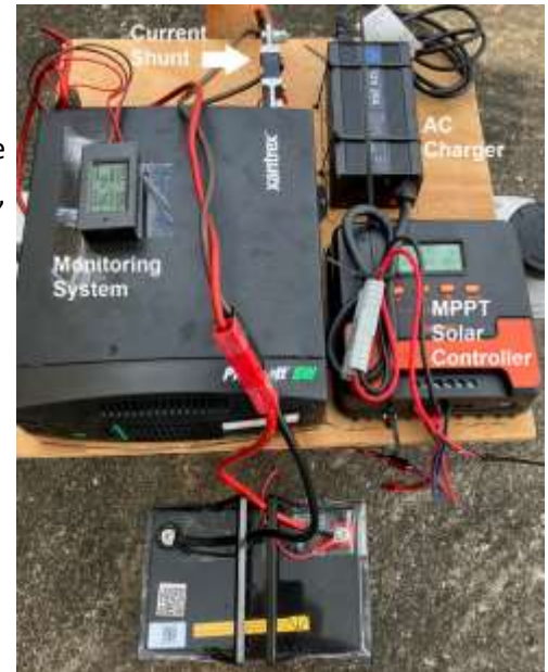
Solar/Inverter System. (Protective insulation not yet on 100AHr battery terminals)
