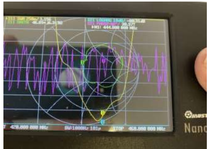
Figure 8: NanoVNA SWR on connected 70 cm Yagi's shows unexpectedly GOOD SWRs. 2:1 is approximately halfway up this display. The SWR at 444.8 MHz is 1.2:1
