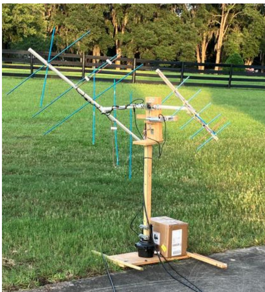
Figure 3 dual axis antenna rotator system with antennas
