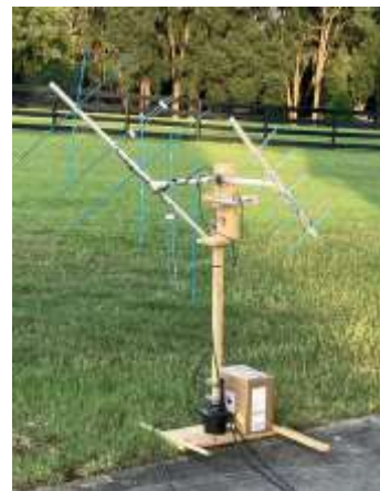
2m/70cm elliptically polarized 2-axis rotation Yagi System for Satellites--Homebrew
