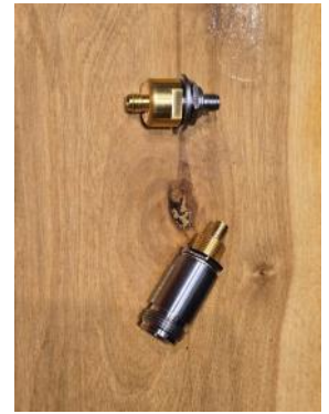
Above are 2.92 mm and SMA to Type N Female-Female bulkhead connectors. The 2.92 mm connector is compatible with SMA and uses an air dielectric instead of Teflon or similar dielectric material. The air type allows the connector to be used at higher frequencies or with lower loss.
