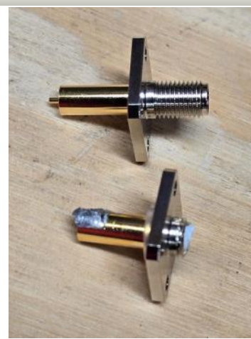
The new and old SMA flange connectors
