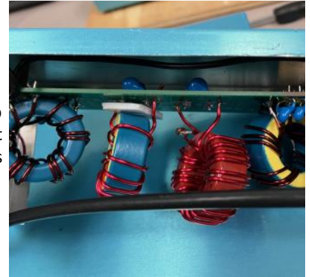
Cold Solder Joint In This Filter Knocked Us Off For an Hour At The Start
