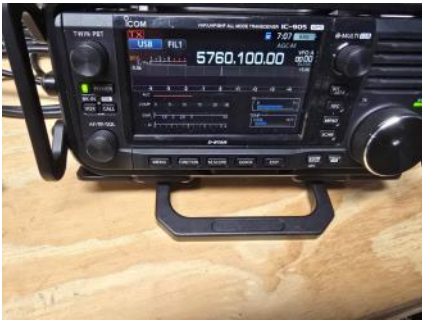
The IC-905 Control Unit showing 5.7601 GHz or 5760.1 MHz.
