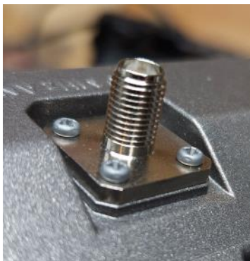
A properly installed and intact SMA flange connector.
