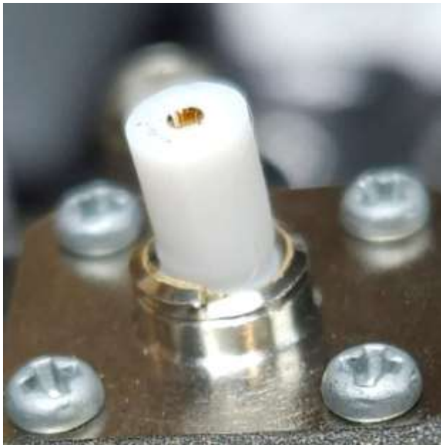
A broken SMA shield on the IC-905 5760 MHz port. I also discovered that a piece of RG-400 broke the SMA bulkhead barrel off the top of the IC-905 and prevented the use of 5760. It had proper strain relief so I am annoyed. I am working on a fix, but I would welcome ideas.
