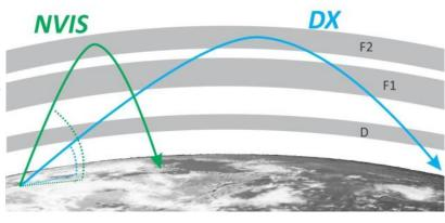
spheric D layer may reduce the signal strength. There is no fundamental difference between NVIS and conventional skywave propagation; the practical distinction arises from different desirable radiation patterns of the antennas (near vertical for NVIS, near horizontal for conventional long-range skywave propagation).
