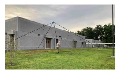
Two types of effective Near Vertical Incidence Skywave (NVIS) antennas. Others exist.
