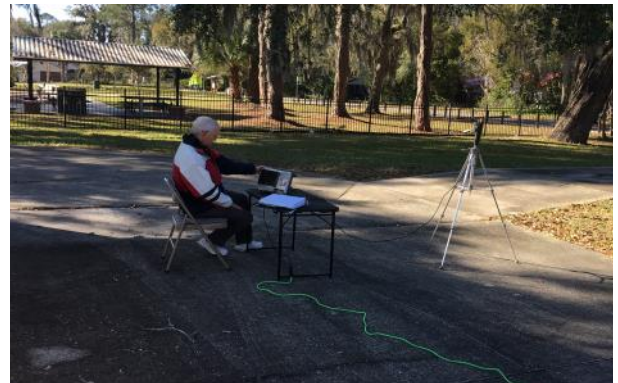
Figure 3. Eric Pleace KO4ZSD monitors the spectrum analyzer with the monitoring antenna close by. The AC power comes from 100+ feet away to further minimize any interference.
