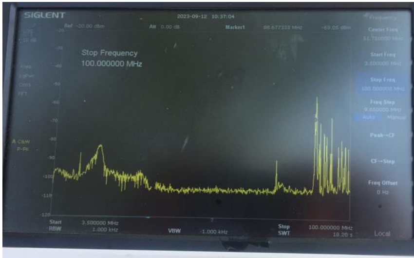
Figure 2: Initial effort at 3.5-100 MHz baseline noise plot. The signals at the right end are FM radio stations; the majority of the apparent noise at the left end of the plot (magnitude -80dBm to -100dBm, frequency 3-18 MHz) is actually created by the inverter power supply.
