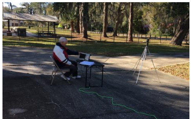
Figure 3. Eric Pleace KO4ZSD monitors the spectrum analyzer with the monitoring antenna close by. The AC power comes from 100+ feet away to further minimize any interference.
