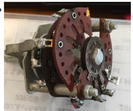
Corroded and broken mode switch.
