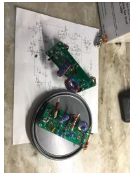
Note unusual coil forms for 10-meter filter...
