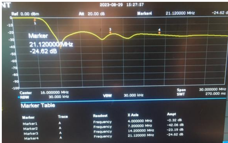
80/160m multiplexer LPF response. A very simple filter, somewhat limited isolation.
