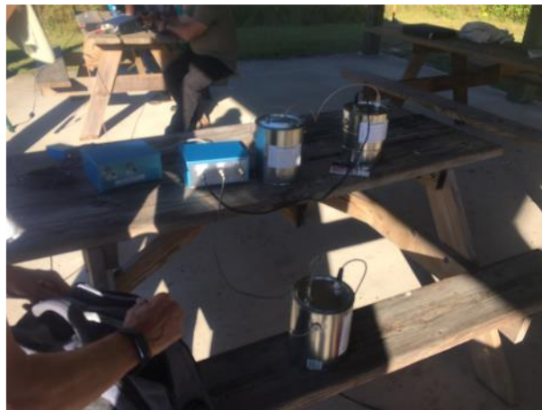
Trial by Fire for our Quintplexor that had us working our choice of 40 / 20 / 15 /10 meters simultaneously out at San
