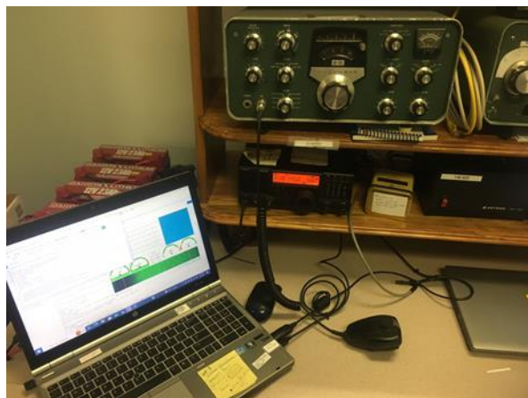
Either of the backup radios can use the sound-interface system -- same pinouts.
