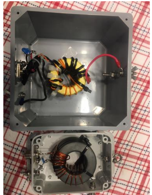
Comparison: homebrew top Balun FT-240-43x3cores; commercial bottom Balun. Both use similar winding technique with a "jump" half-way through the turns. Both 14turns/2turns, primary bifilar twisted.
