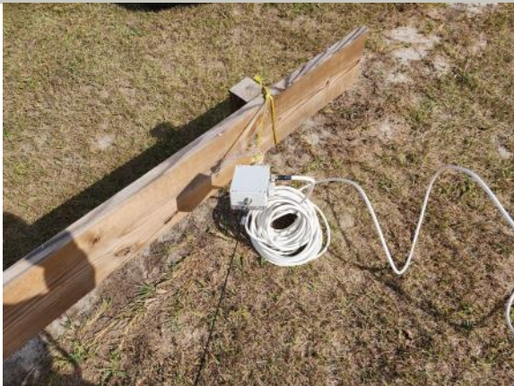
End-fed Half-wave balun and a coaxial choke at Jim K4DBC's POTA/EMCOMM demonstration.
