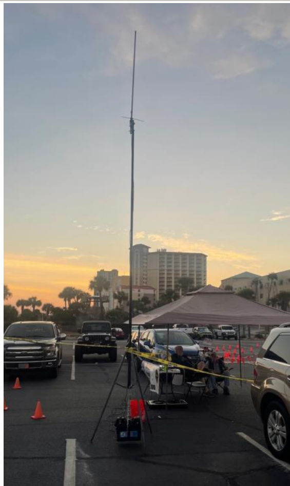
(Right) FFARA Net Control dual band Diamond X30A antenna at 25 feet.
