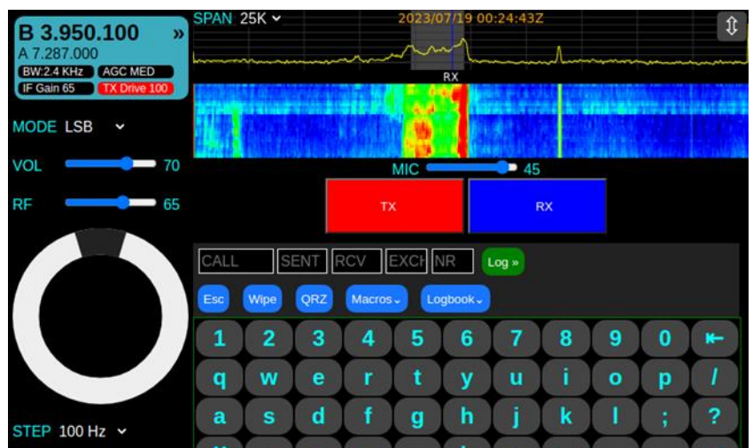
New Web-Based sBitx Interface: Very strong voice signal on 75 meters with onboard keyboard for logging
