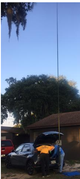
Tim Lynn KD5SSF brought his 30-foot bumper-mounted collapsible fiber-glass vertical. Works via a wire up the center.
