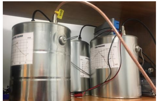
Subject of much mirth in our group, our "paint can filters" follow an ARRL QST article on Butterworth bandpass filters and generally add another 30dB of isolation. Paint cans were an inexpensive shielding.
