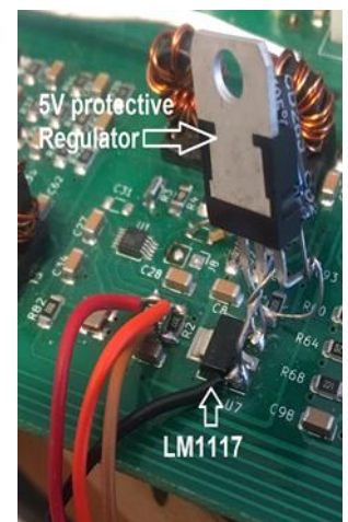
Above—My addition of a 5V pre-regulators to help protect the LMS1117
