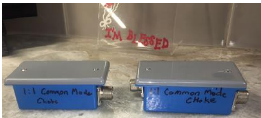
Figure 2: Homebrew 1:1 Choke Baluns
