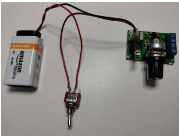
Figure 1: The assembled offset attenuator.
