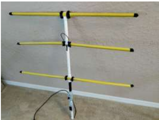
Figure 3. N1JOO's measuring tape yagi.
