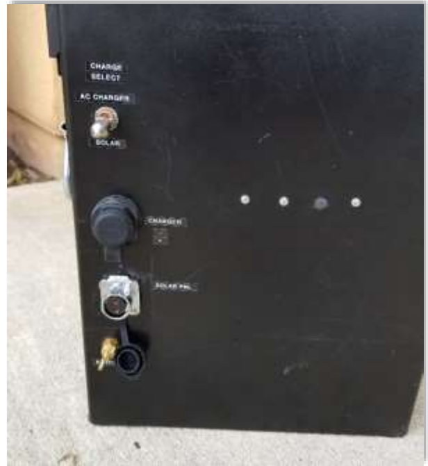
Panel receptacle installed on a solar generator.
