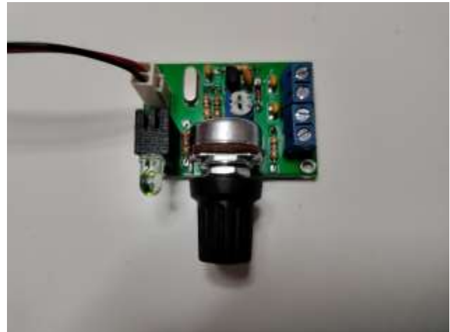
Figure 2: Closeup of the offset attenuator.
