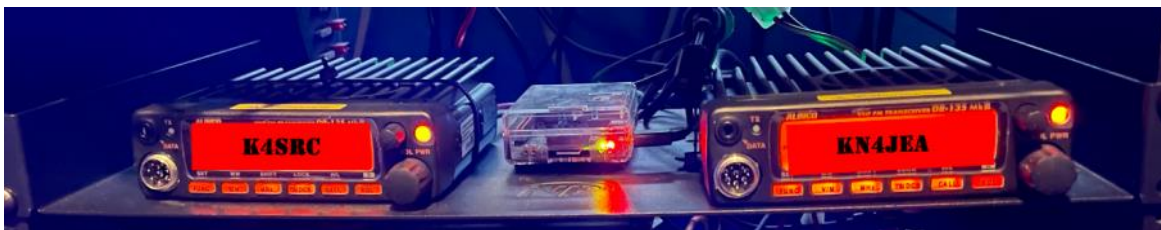
Pictured – K4SRC and KN4JEA linking radios to their respective repeaters and the AllStar Raspberry Pi
