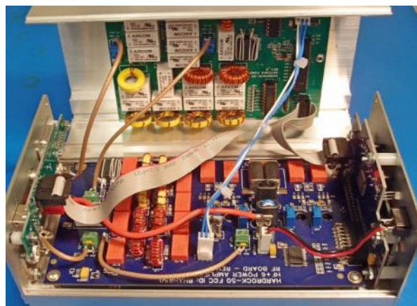
Figure 3: ATU mounted above the RF board. Photo by permission of HobbyPCB.
