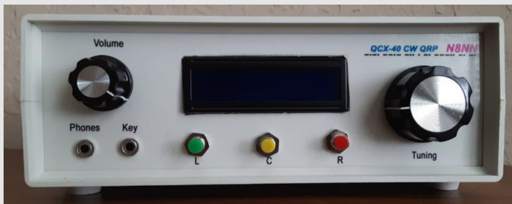
Figure 3: Panel overlay using transparent sticky project paper.
