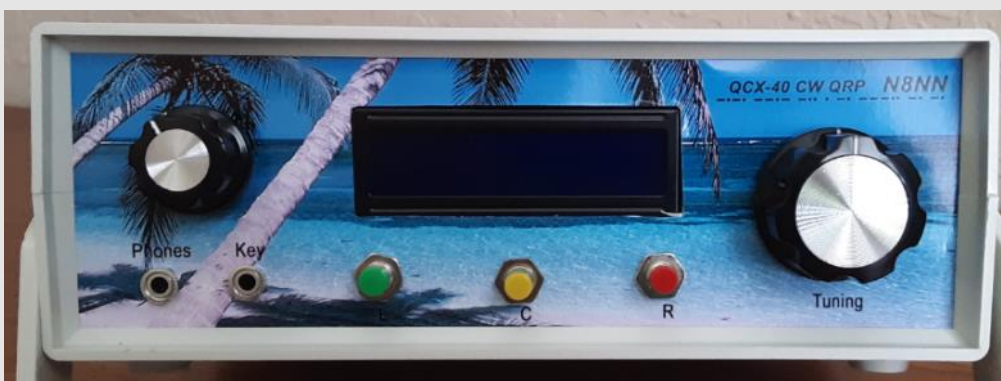
Figure 4: Panel overlay with a tropical flavor printed on glossy photo paper.
