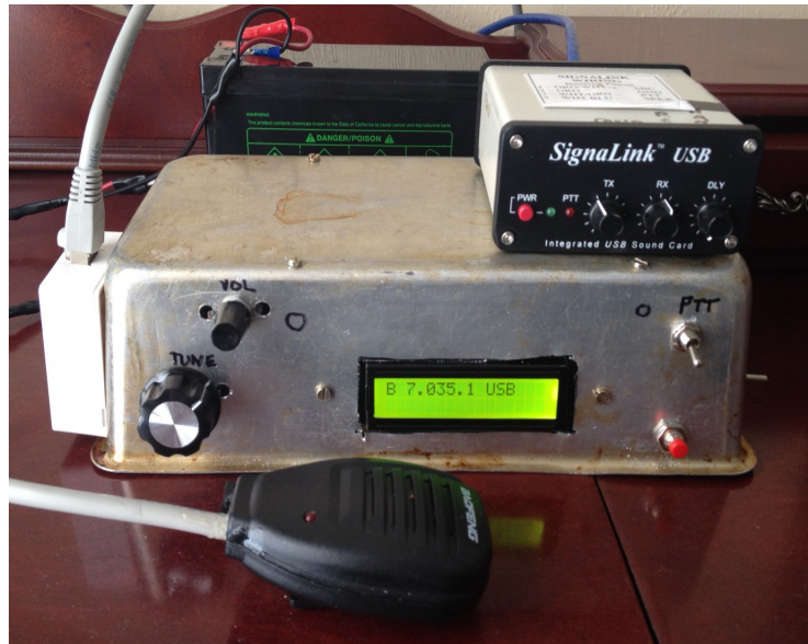
BitX40 enclosed in thrift-shop cake-baking tin; SSB 7-12 watt transceiver can use electret mic or soundcard digital.
