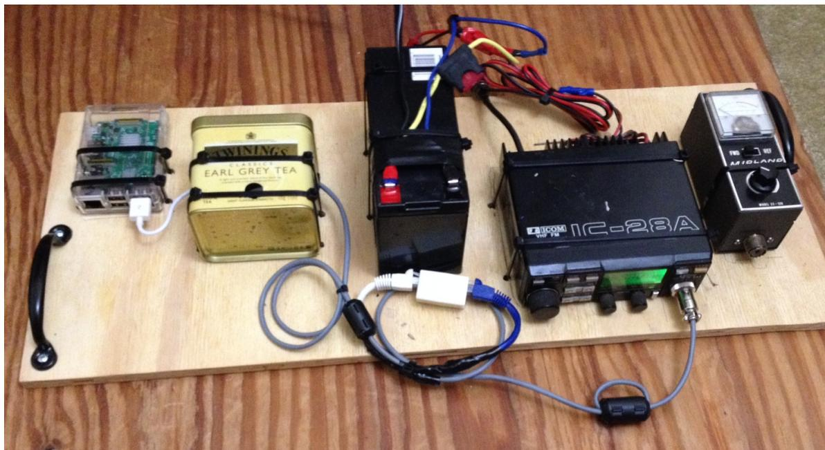
*Prototype Deployable Digital Relay Station -- home made "\$10TNC" soundcard-based interface
