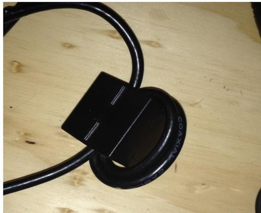
5. **LOOPS** Even simple loops (“scramble-wound”) of signal or coax cables, held in shape with zip ties, can help.
