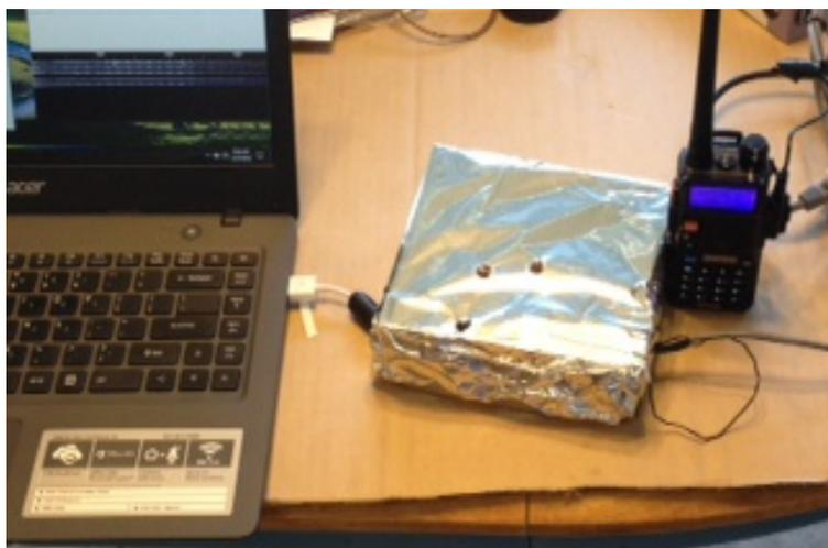
Holes punched to allow access to mic and speaker trimmer pots, and to see the push to talk LED
